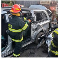
Recently, Haines Falls obtained new Holmatro extrication tools! These electric tools will allow operating more than one tool at a time and the freedom from hydraulic lines.
