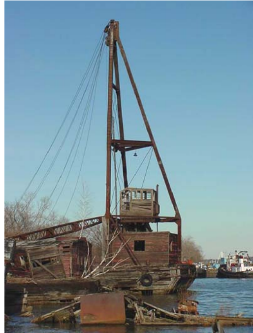
Derrick cranes on barges such as this one are typically used to drive wooden pilings in the construction and rehabilitation of bulkheads.
