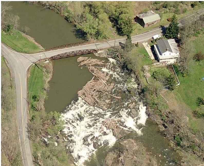
Large woody debris collects on the waterfalls located on the Kaaterskill Creek at Cauterskill Road. Large floods often wash this debris into the Catskill Harbor and can inflict significant damage to docks and boats.
